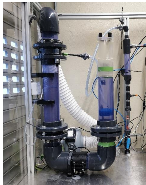
Figure 1. Absorption-Test-Rig for structured packings for liquid-phase DAC.
